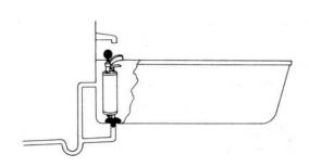
If you're having difficulty with splash back, follow the same basic procedure as for clearing sinks and wash basins. Remove overflow screen and with screwdriver push 8 to 10 inches of thin wet rag down overflow pipe and replace screen.
