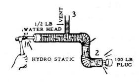
A gauge indicates when the tool has been pumped up to the desired pressure. 98% of the Ram's kinetic force hits the stoppage, while only 2% is spent against the walls of the pipe. The instant impact protects pipes and joints because there's no buildup of pressure in the plumbing system.
