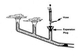
Where there is more than one outlet, always apply Ram where water backs up first. Do not discharge Ram until water appears on floor at next opening. Other drain openings should be covered to protect against splash back.
